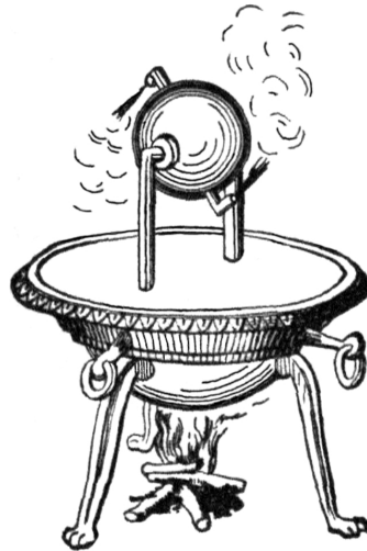
Figure 19.1: The Aeolipile of Hero A small fire boils water and the pressure builds up to ultimately force steam out of angled jets. The flow of steam from the jets rotate the sphere.
